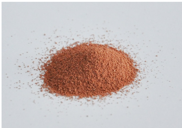
Fig. 1. Powder of copper covered with graphene (Graphene 3D IMP ).
