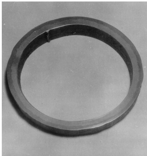
Fig. 2. Cross-section of two pipes connected by explosive welding. Deformation of the pipes (reduction of the internal diameter) was less than 2%.
