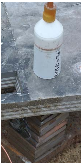
Fig. 1. Test setup for protective capacity of multilayer Ti–Al system.
